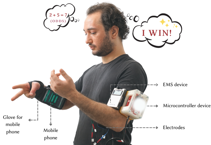
159 160 Figure 3. A participant is wearing the hardware to play “Numbers”. The participant chooses their non-EMS right hand to be “odds”, 161 and the EMS left hand to be “evens”. The with their right non-EMS hand shows a “2”, and their left EMS hand shows a “5” 162 simultaneously, making the sum odd ( 2 + 5 = 7 ). Therefore, the player’s right non-EMS hand wins.
